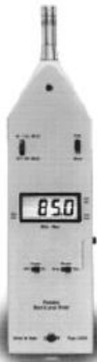
Sound-level meter Measures noise at a moment in time.
